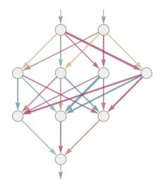
Each "neuron" is effectively set up to evaluate a simple numerical function. And to "use" the network, we simply feed numbers (like our coordinates x and y) in at the top, then have neurons on each layer "evaluate their functions" and feed the results forward through the network—eventually producing the final result at the bottom:
